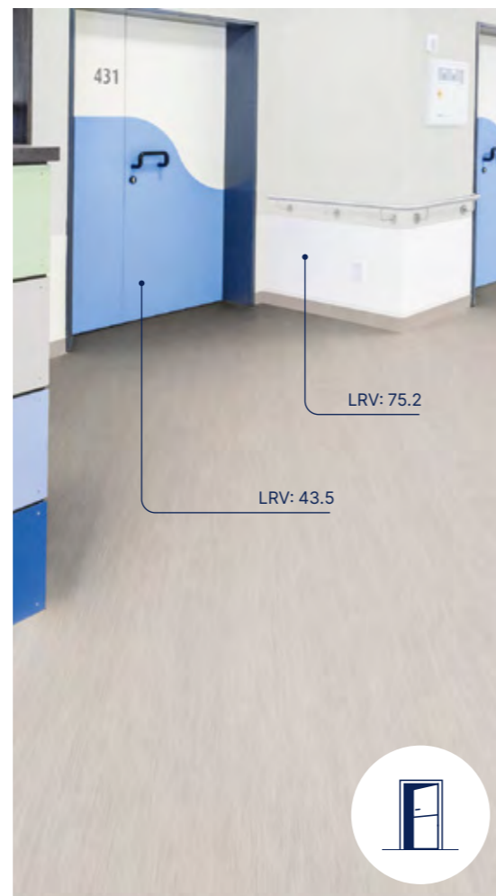
LRV differential of Wall/Door >30 Points = Public Door
