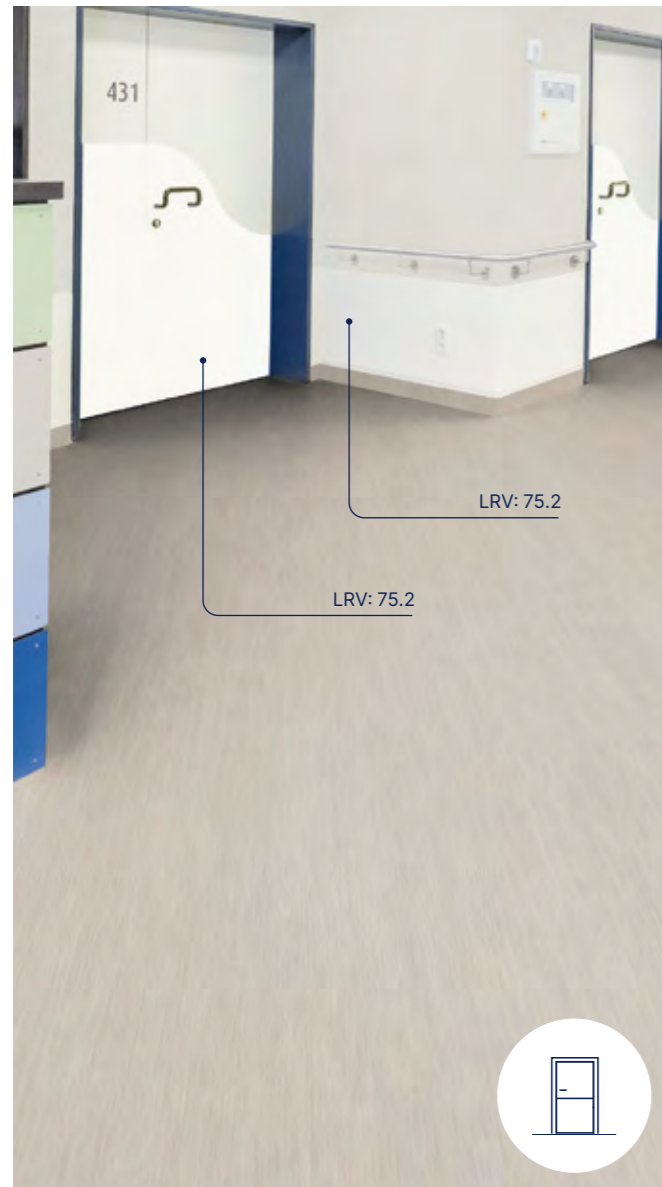
LRV differential of Wall/Door <10 points = Staff Door
